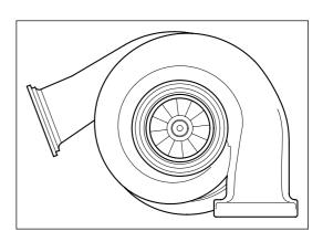
With intake system disconnected from compressor housing, it may be possible to check visually for excess bearing axial and radial clearances.
