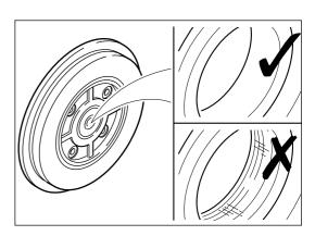
Ensure diffuser/bearing housing sealing ring groove is clean and free from carbon deposits
