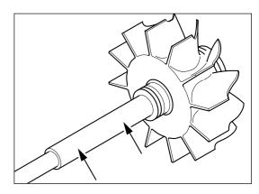
Inspect for cracked, bent or damaged blades.
