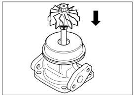
Place assembly on clean flat surface supporting the assembly turbine wheel (6) in a suitable fixture.
