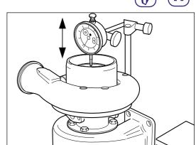
Check the radial movement at compressor impeller nose using a dial gauge.
