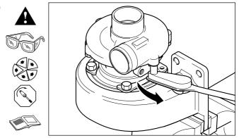
Ensure rotor assembly freely rotates.
