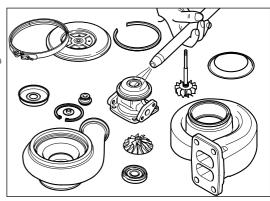
Scale like deposits, if any, must be removed by using a non metallic bristle brush. After loosening the deposits with the brush, wash and dry components as above.
