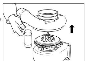
On some turbocharger options, the bearing housing to compressor housing joint is fitted with o-ring seal, compressor (41). This seal should be removed and discarded at this stage
