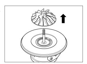
Remove remaining CHRA from fixture and gently slide bearing housing (4) off the assembly turbine wheel (6).
