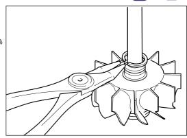
Lubricate the shaft with clean engine oil and insert into the journal bearings. Positively locate the seal ring (13) \* into position and ensure the assembly turbine wheel rotates freely.
