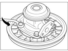
Hold the diffuser (14) flat on a work bench and carefully seperate the bearing housing (4) from the diffuser (14).
