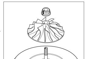
Components that should be included in rotor balance
