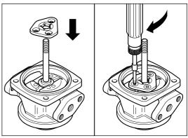
Fit the new piston ring seal (16) \* to the oil slinger (31).
