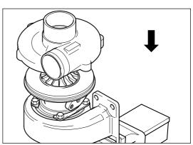
Fit clamp plates, bolts and washers and tighten to value specified in **Service data Sheet**.
