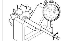
Inspect split ring seal, turbine (13)\* groove walls for wear. If groove width exceeds recommended maximum of 1.69 mm (0.067 in) replace assembly.
