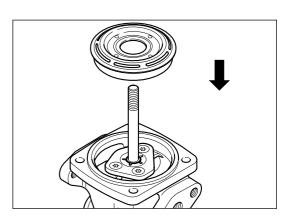
Apply a small amount of engine oil to the diffuser (43) and place the rectangular ring seal (32) into position.
