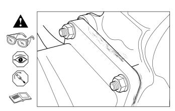
Where practical remove exhaust system pipework to check exhaust system connecting profile for fretting damage.
