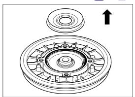
Remove and discard rectangular ring seal (32) \* Remove the oil slinger (31).
