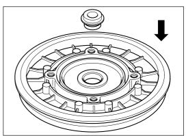
Install the oil baffle (33) into the bearing housing (4).
