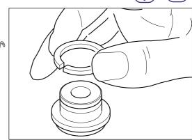
Using clean engine oil, lubricate the oil slinger (31) and install into the diffuser (43).
