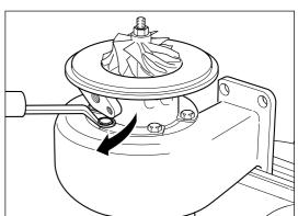
Check thrust clearance using a dial gauge. Ensure clearance is within MIN/MAX values shown on **Service Data Sheet**.
