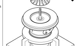
Align the balance marks scribed on shaft and compressor wheel.
