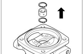
Turn the bearing housing over and repeat the process of retaining ring (64) \* and bearing (11) \* removal at turbine end.
