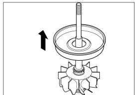
Carefully remove the split ring seal, turbine (13) \*.
