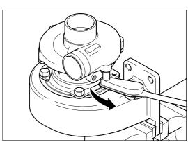
Ensure rotor assembly freely rotates.
