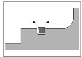
Inspect the bearing journals for excessive scratches and wear. Where scratching is excessive or where either journal diameter is less than the recommended minimum of 10.97 mm (0.43 in) replace the assembly.
