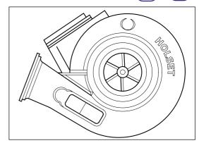
Where practical, check for cracked, bent or damaged turbine wheel blades.
