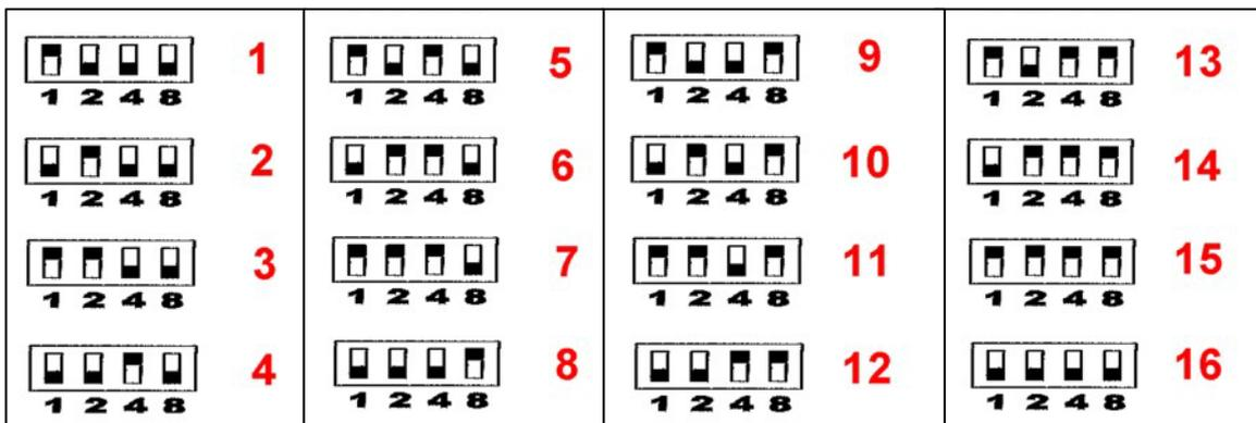
Fig. 11: Compressor Wheel Blade Setting Diagram
