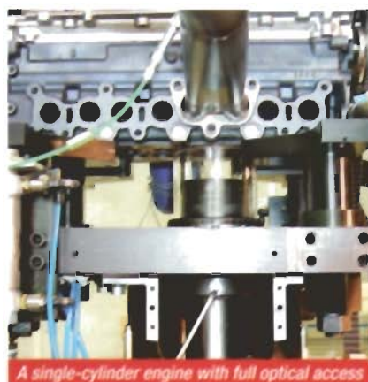
A single-cylinder engine with full optical access
