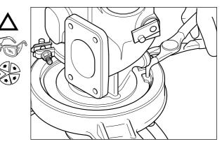
Tap ends of retaining ring with hammer and drift to ensure that the retaining ring is properly located into its groove in the bearing housing.
