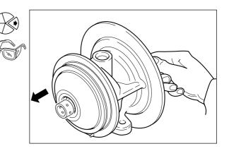
Pull the spring (127) out on a finger from the turbine end.
