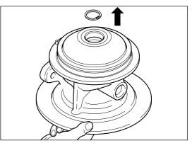
With a finger push the spring (127) from the compressor end to force the journal bearing (11) \* out. Discard bearing.
