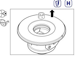
Turn the bearing housing over. Using circlip pliers, Part No. 56664, remove and discard the remaining retaining ring (64)  $\star$ .
