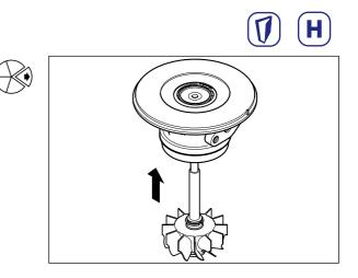
Remove remaining CHRA from fixture and gently slide bearing housing (4) off the assembly turbine wheel (6).
