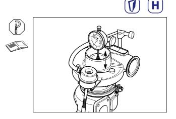
Check the radial movement at compressor impeller nose using a dial gauge.
