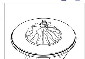
Inspect internal profile of compressor housing for scoring damage due to possible contact with compressor wheel. Check compressor housing retaining ring groove is free from deposits and is not worn.
