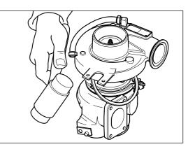
The bearing housing to compressor housing joint is fitted with 0-ring seal, compressor (41). This seal should be removed and discarded at this stage.
