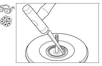
Ensure that back face of compressor wheel (7) is clean and free from damage. Install on to the shaft.
