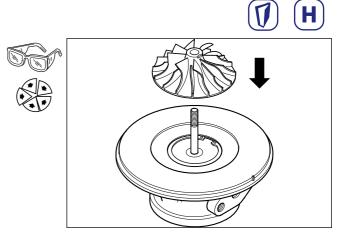
Align the balance marks scribed on shaft and compressor wheel.
