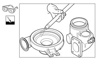
Scale like deposits, if any, must be removed by using a bristle brush. After removing the deposits , re-wash and dry the components.
