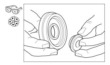
Install the oil baffle (33) \* into the oil seal plate (43).
