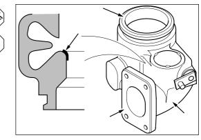
After washing and bead blasting the wastegate valve mechanism may remain seized or stiff to operate. If so, soak the mechanism in penetrating oil for approximately 20 minutes or a period of time recommended by the oil manufacturer.
