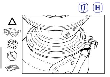
Check thrust clearance using a dial gauge. Ensure clearance is within MIN/MAX values shown on *Service Data Sheet*.
