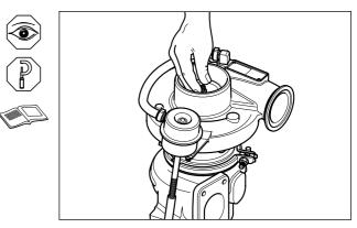
If it is possible to check for wastegate actuator rod movement and air leakage on engine, follow the checking procedure described later in *Wastegate Actuator Checks*.
