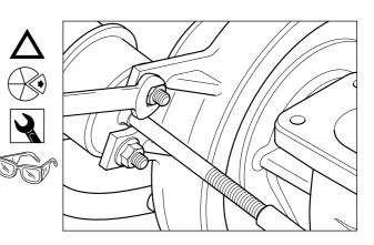
Lift the actuator away from the bracket until the studs clear the location holes.
