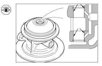
Check oil seal plate, retaining ring groove does not exceed a maximum width dimension of 2 mm (0.079 in).
