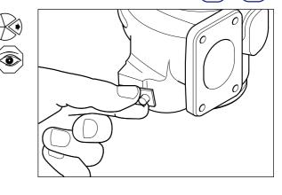
Access to the wastegate valve from the exhaust outlet is limited but, with care, soaking with penetrating oil is possible.
