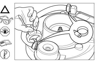
New pre-set actuator kits may be supplied with a tamper resistant break off nut instead of a jam nut to secure the end link in its correct pre-set position. To install a tamper resistant actuator
