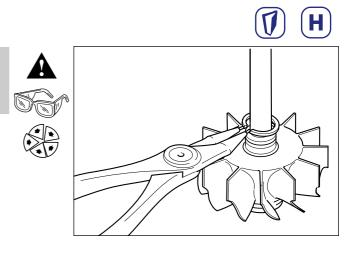
Lubricate the shaft with clean engine oil and insert into the journal bearings. Positively locate the seal ring (13) \* into position and ensure the assembly turbine wheel rotates freely.
