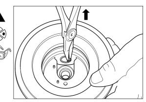
With a finger remove the journal bearing (11) \* from the compressor end and discard.
