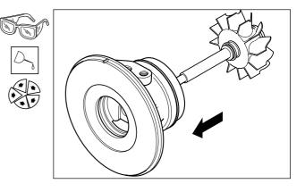
Place assembly on clean flat surface supporting the assembly turbine wheel (6) in a suitable fixture.
