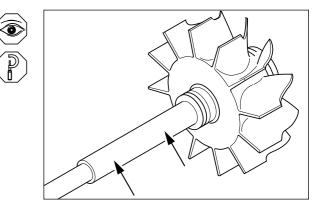
Inspect for cracked, bent or damaged blades.
