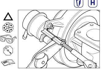
Re-fit end link to the lever arm pivot pin. Fit new e-clip using special tool Part No. 4027204 to retain rod end on pin.
