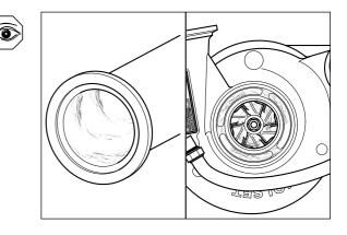
Always refer to *Cleaning of Housings* to clean housing. Rotor components can be cleaned using a bristle brush.
