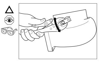
Check the wastegate lever arm for evidence of rubbing or cracking. Replace with a new turbine housing if damage is visible.
