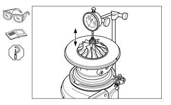
Check compressor end radial movement using a dial gauge. Ensure clearance lies within MIN/MAX TIR (Total Indicator Reading) values shown on *Service Data Sheet*.
