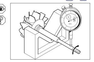
Inspect split ring seal, turbine  $(13)^*$  groove walls for wear. If groove width exceeds recommended maximum of 1.69 mm (0.067 in) replace assembly.
