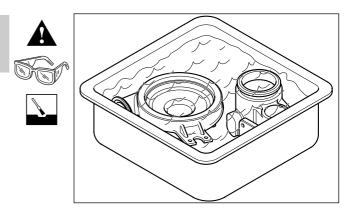
Dry the components using compressed air.
