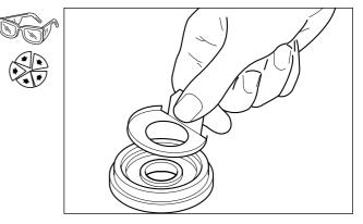
Align the tongue of the oil baffle with the aperture in the bearing housing and install the seal plate assembly.
