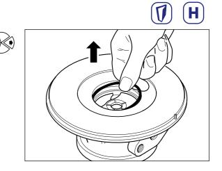
Remove the thrust bearing (12) \* and discard.
