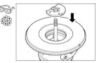
Insert the O-ring seal, bearing housing (32) \*.
