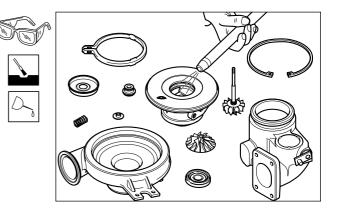
Scale like deposits, if any, must be removed by using a bristle brush. After loosening the deposits with the brush, wash and dry components as above.
