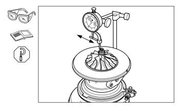
To refit compressor housing place the turbine and bearing housing assembly on clean surface. Carefully locate the compressor housing over the compressor wheel and locate on the bearing housing spigot.
