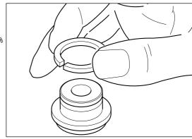
Install oil slinger (31) into oil seal plate (43).
