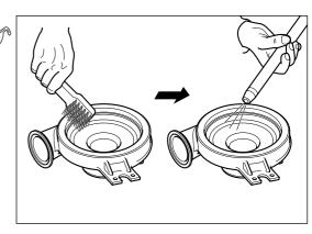
It is permissible to bead blast the turbine housing if chemical and brush cleaning is not effective.
