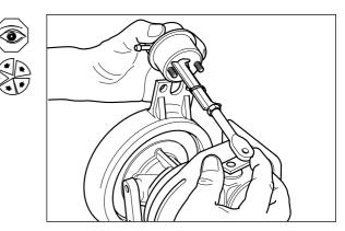
To adjust the length of the actuator assembly, remove from the turbocharger. Rotate the end link (76) to shorten or lengthen the rod as appropriate. Re-fit, until the underside of the pre-set actuator (73) will just fit over the bracket mounting face with less than 0.5 mm (0.020 in) gap.
