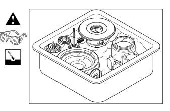
Dry the components using compressed air.
