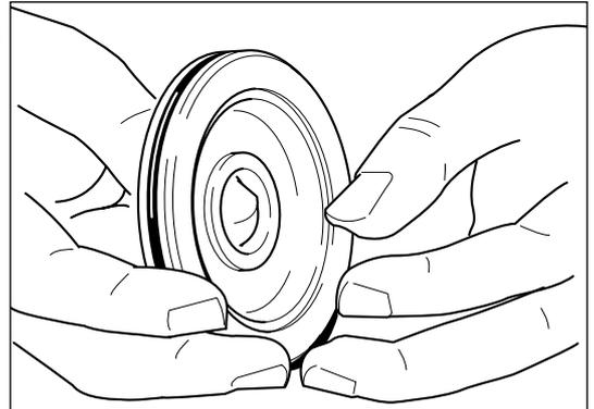
Fit new split ring seal/seals, compressor (16)\* to oil slinger (31).
