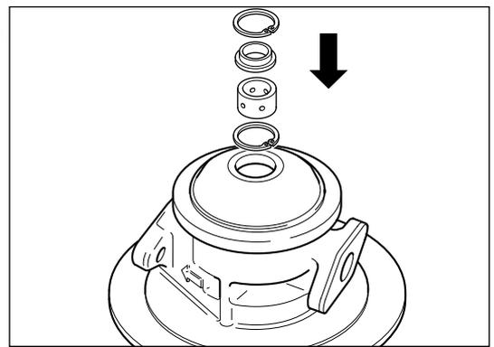
Fit the outer retaining ring (64)\* with the bevelled edge facing the bearing.
