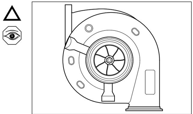
Where practical, check for cracked, bent or damaged turbine wheel blades.
