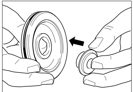
Press fit oil baffle (33)\* into oil seal plate (43).
