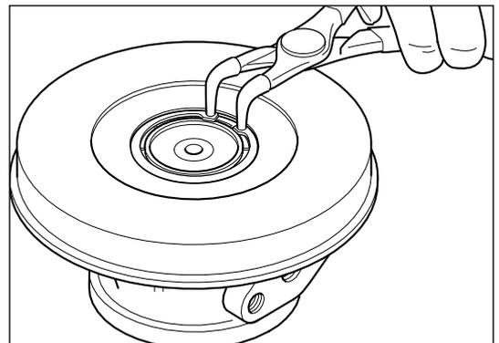
It is practical to use free hand to contain disassembled ring whilst releasing pliers.
