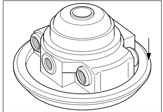
Check oil seal plate, retaining ring groove does not exceed a maximum width dimension of: 2 mm (0.079 in).
