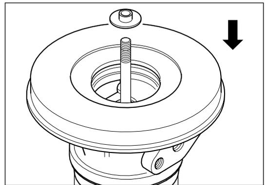
Apply clean engine oil to installed thrust collar (36) and insert thrust bearing (12)\* on to its location pins.
