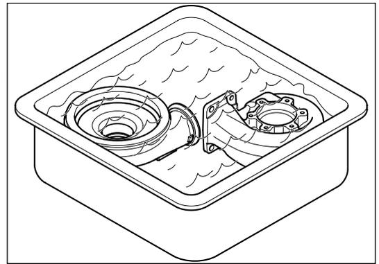
Dry the components using compressed air.
