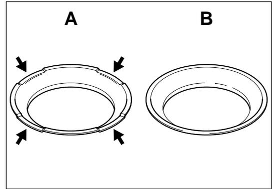
**Caution** When removing the inlet baffle retaining ring, be careful not to damage the compressor wheel with the screw driver. Use a rag or rubber bung to protect the wheel.
