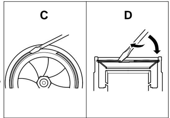
Push the screwdriver in an anti-clockwise (counter-clockwise) direction to force the retaining ring out of the groove. Remove the retaining ring.
