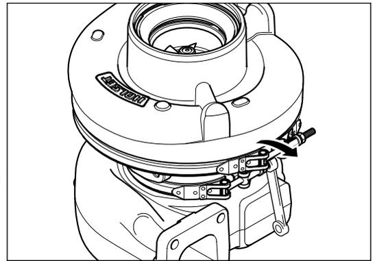
Using a soft hammer, tap turbine housing down against soft bench surface. As bearing housing and compressor housing assembly comes loose gently lift it out of turbine housing engagement
