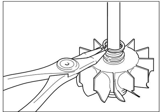
Where fitted, use circlip pliers Part No. 56663 to remove heat shield retaining ring (95)
