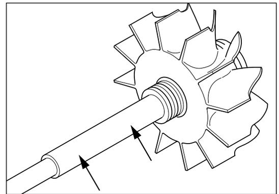
Inspect for cracked, bent or damaged blades.
