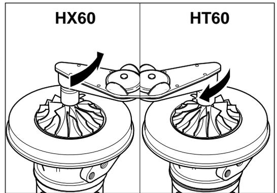
Place turbine housing (5) on a clean surface. Place V-band clamp loosely into position on the turbine housing. Carefully slide CHRA (2) assembly into the turbine housing.
