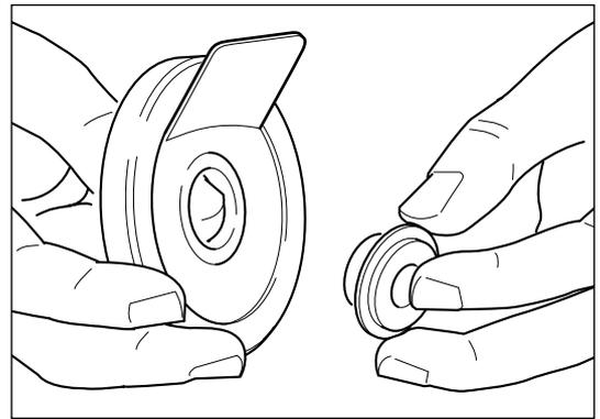
Using a small screwdriver, release oil baffle (33)\* from its light fit location in the oil seal plate (43) and discard.
