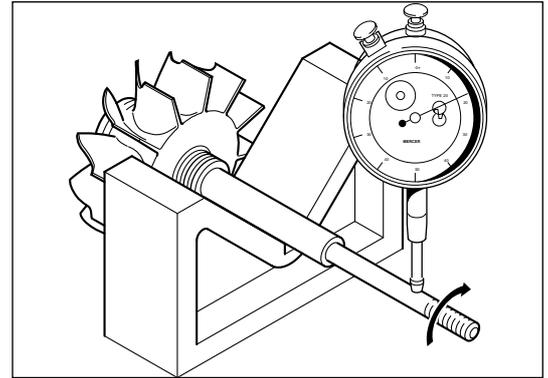
Inspect split ring seal, turbine (13)\* groove walls for wear. If groove width exceeds recommended maximum of 1.90 mm (.075 in) replace assembly.
