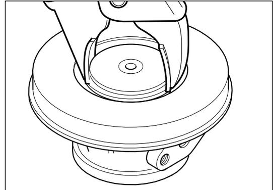
Disassemble oil seal plate (43) assembly by first removing oil slinger (31).
