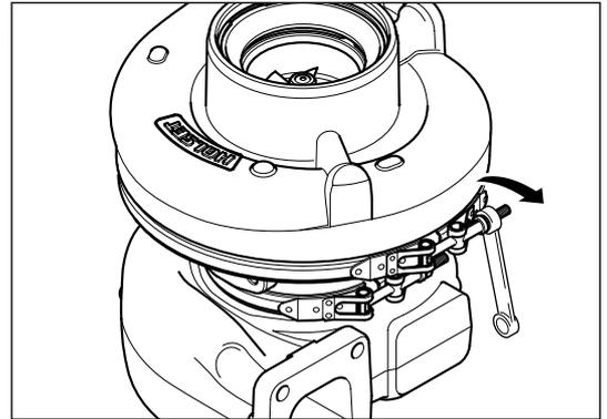
Ensure rotor assembly freely rotates.
