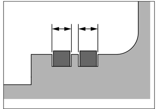
Inspect the bearing journals for excessive scratches and wear. Where scratching is excessive or where either journal diameter is less than the recommended minimum of 14.25 mm (0.561 in) replace the assembly.
