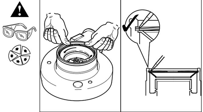
Place the turbine and bearing housing assembly on a clean surface. To refit compressor housing, loosely fit V-band clamp. Carefully locate the compressor housing over the compressor wheel.
