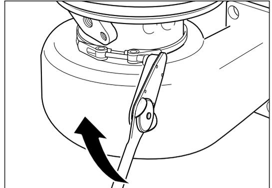
Ensure rotor assembly freely rotates.
