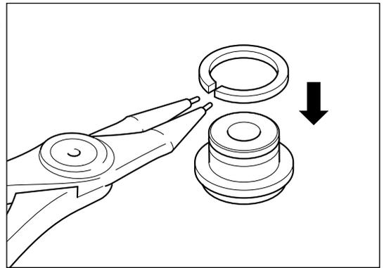
Lubricate oil slinger (31) and insert into oil seal plate (43).
