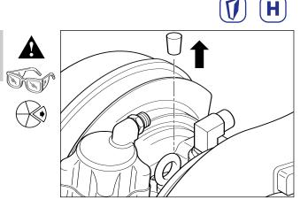
Prior to inserting speed sensor ensure it is clean and unable to collect metal particles as it is inserted. Ensure o-ring seal is in position on sensor body.
