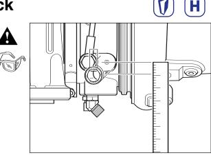
Ensure hose from dry regulated air supply is properly secured to actuator air inlet.
