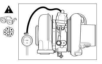
Apply 300 kPa (43.5 lbf/in<sup>2</sup>) maximum 450 kPa (65 lbf/in<sup>2</sup>) air pressure until actuator is moving freely over whole stroke.
