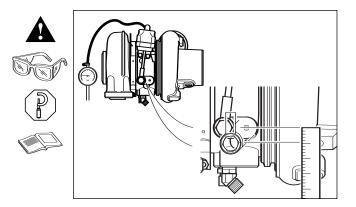
Whilst air pressure is still applied at 300 kPa (43.5 lbf/in<sup>2</sup>) check actuator for leaks. Use soapy water and small brush. Small bubbles will appear if actuator is leaking. If actuator is leaking, it must be removed by reference to *VG Actuator Removal*.
