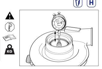
Check radial movement at compressor impeller nose using dial gauge.
