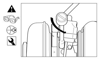
Connect clean dry regulated air supply to actuator air inlet and apply 200 kPa (29 lbf/in<sup>2</sup>) pressure to release actuator pre-load between bracket and lever.
